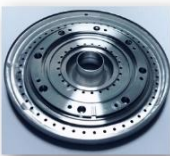
Anode backplate Plateau (304L inox)
